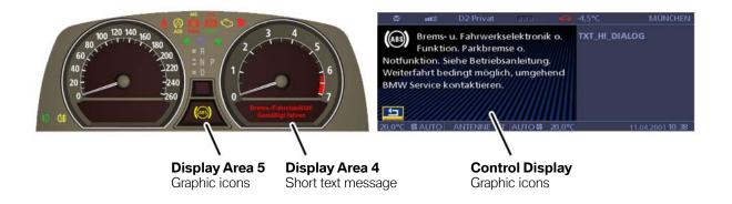
The variable graphic icons are displayed in yellow or red in display area 5 below the gear display. Normally, the time and outside temperature are displayed in this area, these can be overwritten by the Check Control where required.
